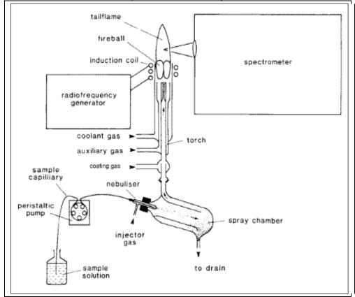
The most common sample delivery system consists of a peristaltic pump and capillary tube to deliver a constant flow of analyte liquid into a nebuliser.
