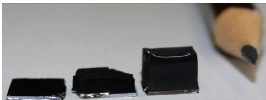
Millimeter-tall carpets of crystalline and vertically aligned carbon nanotubes synthesized on silicon substrates
